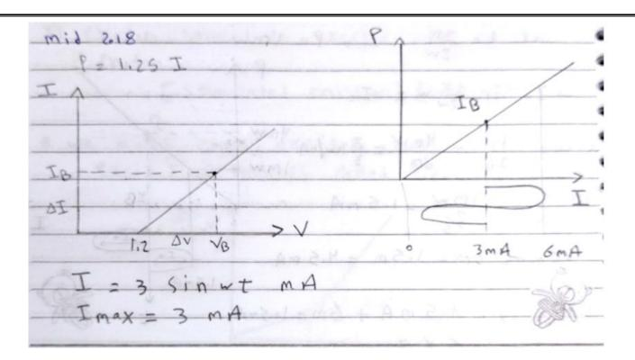
$P = 1.25 \Gamma = 1.25 \times 3m = 1.$   $\Delta \Gamma = 16m \Delta V$   $3m = 16m \Delta V$   $VB = \Delta V + 1.2 = 1.39V$   $RS = \frac{3-1.39}{3m} = 537-2$
